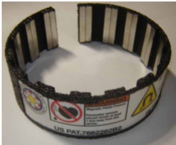
Figure 3.1: Magnetic Array Filter (MAF)
